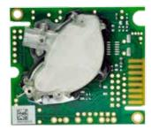
CO<sub>2</sub> Engine<sup>®</sup> LP is a low-power module that fits in any application where power consumption is important to keep at a minimum without sacrificing performance. The platform is designed for integration into host apparatus, such as battery operated products. The module also measures temperature, and humidity is an option.
