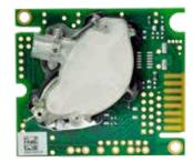
CO<sub>2</sub> Engine® ELG is suitable for low power applications as the unit can be put into sleep-mode between measurements. The sensor measures and stores records of environmental parameters such as CO<sub>2</sub>, RH and temperature.
