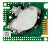
CO<sub>2</sub> Engine® K30 FR is a high performance CO<sub>2</sub> sensor module optimized for fast response time. The sample cell is well protected by a particle filter and is designed for fast diffusion without any need for external pump. In addition, there is a tube inlet to be able to feed on-line test gas through the sensor.
