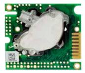
CO<sub>2</sub> Engine<sup>®</sup> K30 can be customized for a variety of sensing and control applications. The platform is designed to be an OEM module for built-in applications in a host apparatus. K30 is a flexible product with 2 analog outputs and 2 digital outputs that can be configured with SADK or other custom software.
