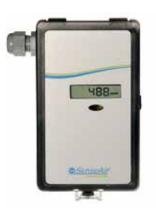
aSENSE™ MIII DISP IS a controller with Dulit-in sensors to monitor carbon dioxide and carbon monoxide simultaneously. With these parameters, the programmable unit can for example control ventilation rates and generate alarm signals. The sensor can be configured with the UIP Software.
