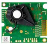
The CO<sub>2</sub> Engine® ICB platform can be customized for a variety of sensing, control and alarm applications. This platform is designed to be an OEM module for built-in applications in a host apparatus.
