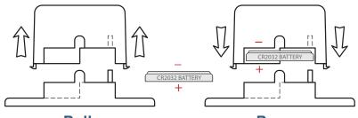
Pull (sensor away from base) Press (sensor back into base)
