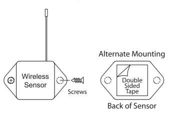
In order for your wireless sensors to work optimally, you should orient all antennas for your sensors and gateway(s) the same direction (typically vertical). Also sensors must be at least 3 ft. away from other sensors and the wireless gateway in order to function properly.
