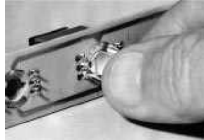
2. A 1/8-turn applied clockwise to the receptacle locks it in the printed wiring board and establishes the electrical connection.
