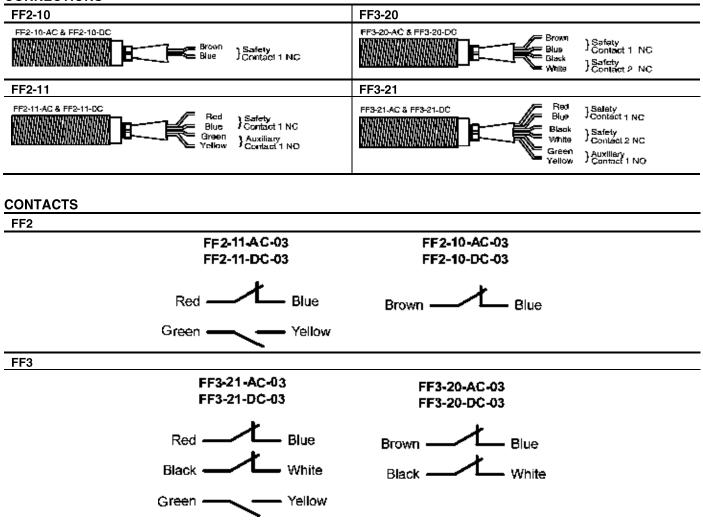
NOTE: Contact configurations show under closed condition for guard device.
