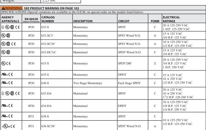
Supplied with 8 ft. 14/3 cord and 3 prong series plug. Green lead grounded. <sup>2</sup>Supplied with 8 ft. 16/3 cord, wired N.O. with green lead grounded. <sup>3</sup>DB Double Break models must be wired to equal voltage sources and the same polarity. The loads should be on the same sides of the line. <sup>4</sup>Supplied with 6 ft. 18/3 cord.
